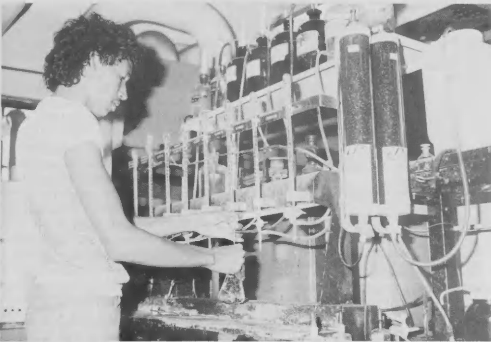
Beltran Lugo inspects a heating oil sample for mercaptan sulphur.
